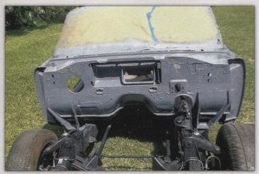
After the body was bolted back on the frame to have the replacement The replacement 318-cu.in. V-8 engine was sent to Lake Park Auto floor pans precisely aligned, it was lifted off again in order to be sprayed with a single coat of Eastwood's Encapsulator Epoxy, followed by two coats of urethane primer/sealer.
