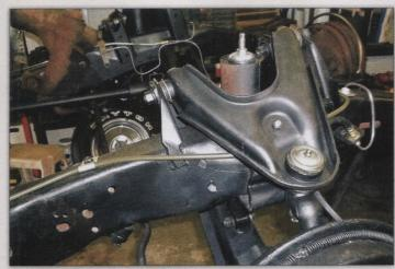
Every wearing component, such as ball joints, tie-rods, bushings, bearings, seals and shocks was replaced with a new part. The old rusted gas and brake lines, and brake flex hoses, were also replaced, including the little brackets that hold them onto the frame.
