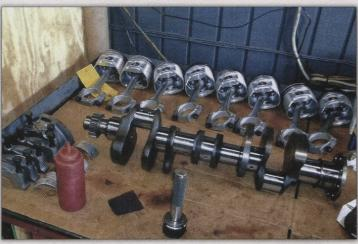
Machine Shop in nearby Lake Park to be machined and rebuilt. The block was bored .030-over and fitted with new pistons; the crankshaft was cut .010, polished and balanced for smooth operation.
