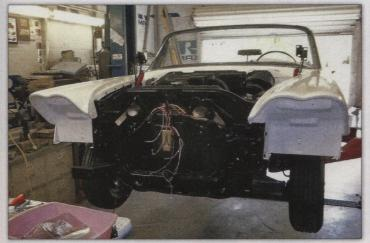
This is the period during a restoration when progress slows down, because you need to take extra care in bolting the restored components back in place without damaging them or chipping the new paint. With the fenders on, next came the headlamps and grille.
