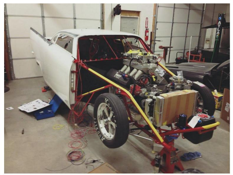
The chassis is a 6.00 certified piece from GPS with <u>Strange Engineering</u> brakes, struts, shocks, axles, and center section. The Fab-9 rearend was custom built by GPS Race Cars in-house for the car. For electronics, Rone opted to use <u>MSD</u> and K&R parts to keep the fire in the pipes. A set of Sanders wheels and Hoosier tires keep the Saratoga rolling down the track.
