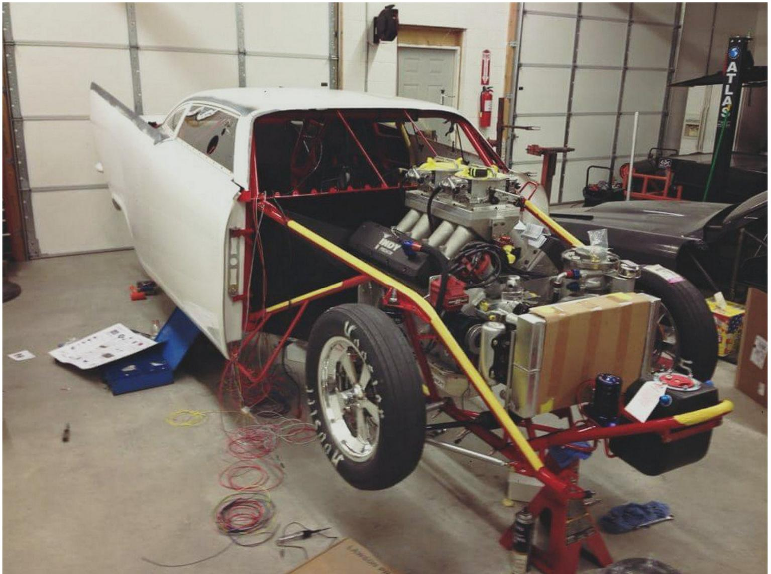
The chassis is a 6.00 certified piece from GPS with [Strange Engineering](#) brakes, struts, shocks, axles, and center section. The Fab-9 rearend was custom built by GPS Race Cars in-house for the car. For electronics, Rone opted to use [MSD](#) and K&R parts to keep the fire in the pipes. A set of Sanders wheels and Hoosier tires keep the Saratoga rolling down the track.
