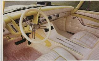
Every corner of the cockpit has been rebuilt. Bob Divine out of Martinez, California, constructed and upholstered the custom bucket seats and rear bench. The white vinyl upholstery with chartreuse piping combines tuck 'n' roll and button-tuft patterns, and extends across the dash. Divine also created the center console and handmade headliner and finished the trunk.
